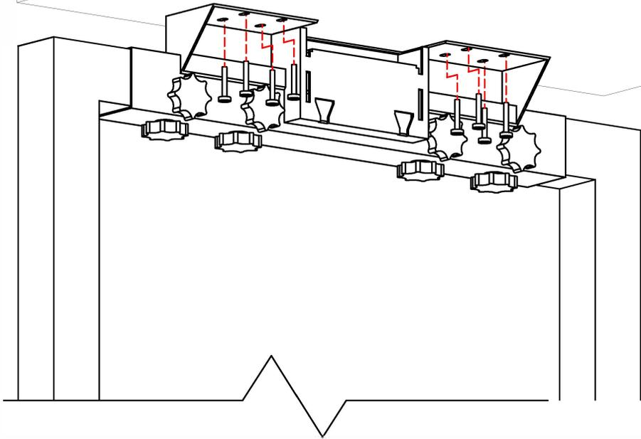
5. IF USING LEG ON RETURN WORKSURFACE REFER TO FIG. A AND ATTACH USING HARDWARE PROVIDED. (REFER TO LAYOUT FOR HANDEDNESS)
