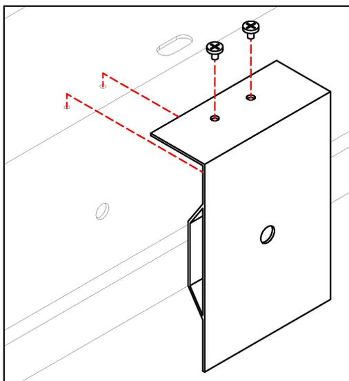
5. IF SCREEN IS REQUIRED, ATTACH BRACKETS TO TROUGH WITH HARDWARE PROVIDED.
