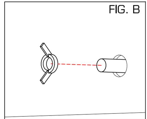
6. IF SCREEN WAS ORDERED, ALIGN HOLES ON SCREEN WITH HOLES ON SCREEN BRACKETS AND ATTACH USING SCREW (FIG. A) AND WINGNUT (FIG. B).
