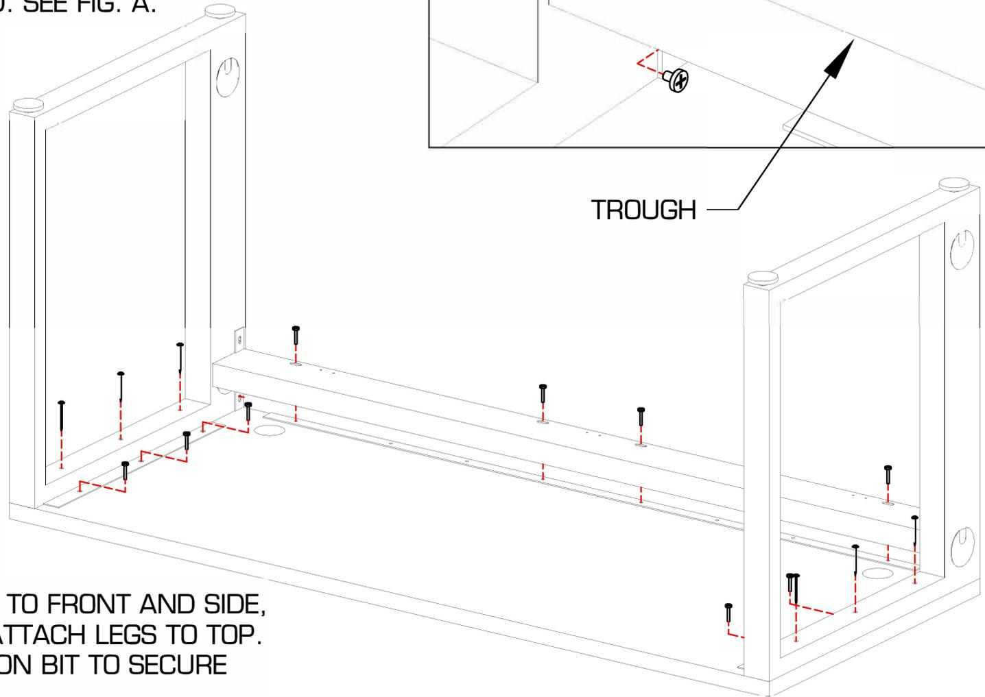
3. ALIGN RIGHT AND LEFT LEGS TO FRONT AND SIDE, USE PROVIDED SCREWS TO ATTACH LEGS TO TOP. USE 6" OR GREATER EXTENSION BIT TO SECURE TROUGH TO WORKSURFACE.
