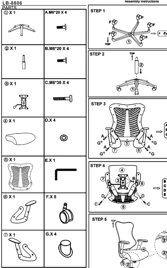
EVERY 6 MONTHS, PLEASE MAKE SURE ALLBOLTS, SCREWS AND KNOBS ARE FULLY TIGHTENED TO **ENSURE STABILITY.**
