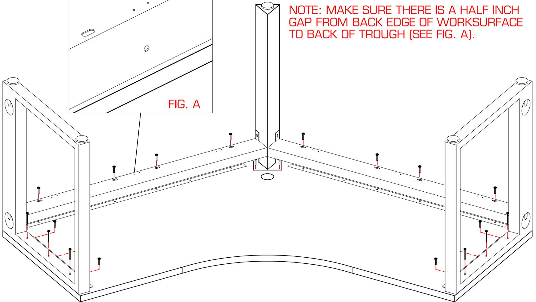
6. IF SCREENS WERE ORDERED WITH STATION, ATTACH SCREEN BRACKETS TO TROUGH AS SHOWN BELOW USING HARDWARE PROVIDED.
